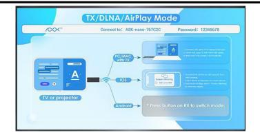
1) When using Windows computer to project, plug TX HDMI, then the screen of computer can be cast to the big display after several seconds;
