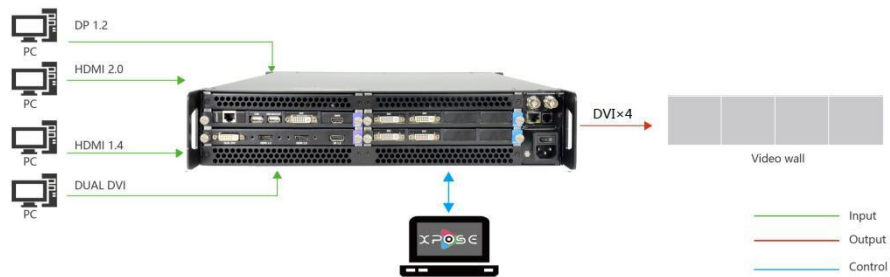
FLEX 4ml System Connection Diagram
